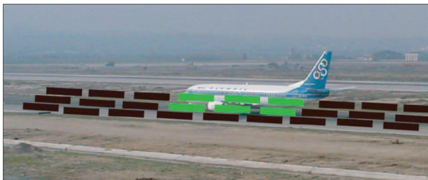
Figure 3. A camera's field of view and detector configuration. The aircraft indicates its presence by activating detectors, which then appear bright green on the system display (shown in light gray here).
